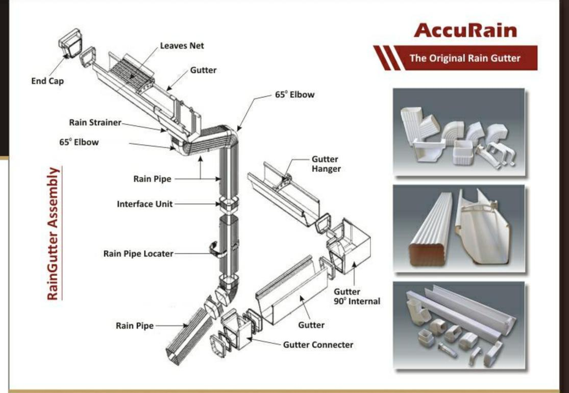
When you choose our AccuRain - RainGutter system, you are sure to find a perfect style gutter with full range of original accessories and fittings. These gutters are manufactured from high impact, high gloss uPVC for a long lasting weather proof performance.
