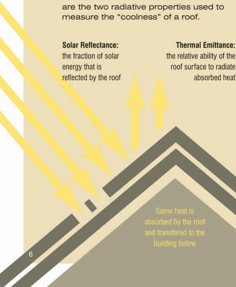
Some heat is absorbed by the roof and transferred to the building below
